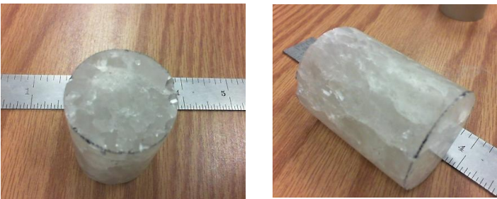
Halite cylindrical sample ( D=36.84\text{mm} , L=50.36\text{mm} )
